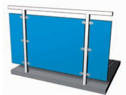
Visible sectional fixing to the balustrade supports
