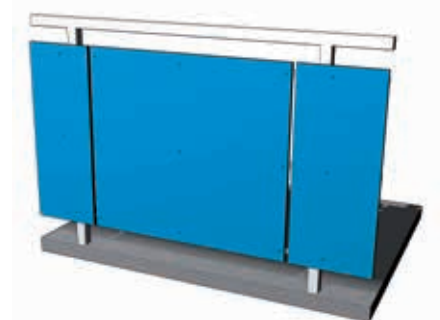
Visible sectional fixing to the balustrade supports with "Z"-profiles
