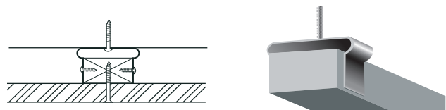
Image 21: Spring clamps for fixing beams with exterior cladding to the load-bearing construction.
