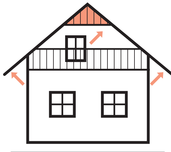
Image 16: Roof covering. In this case the protected exterior is under wood as a condition of use in moisture class 2.
